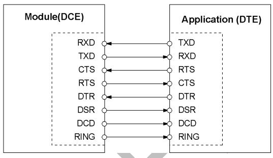
The RS-232 Transceivers can be used to connect the MC509 module to the RS-232-C interface. In this connection, the complementary metal oxide semiconductor (COMS) level and the Electronic Industries Association (EIA) level are converted mutually.
